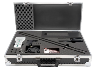
Airbus HFEC Inspection Kit 1.837.69-0038
